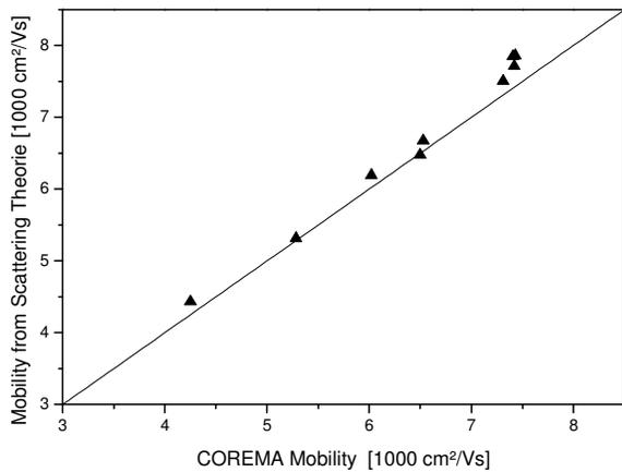
Fig.5 Comparison of mobility data obtained by magnetoconductive measurement with drift mobility obtained from ionized impurity scattering
