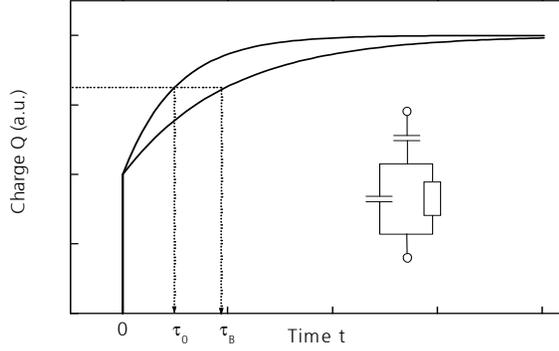
Fig. 2 Charge transients observed after application of a voltage step. The influence of the magnetic field  $B$  is indicated. The insert shows the equivalent circuit of the capacitive probe.
