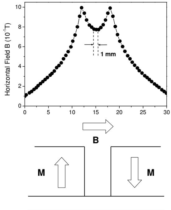
Fig. 6 Schematic representation of the permanent magnets supplying the horizontal magnetic field B. The upper part shows the calculated horizontal magnetic field in the plane 0.5 mm above the permanent magnets (data courtesy Vacuumschmelze ).
